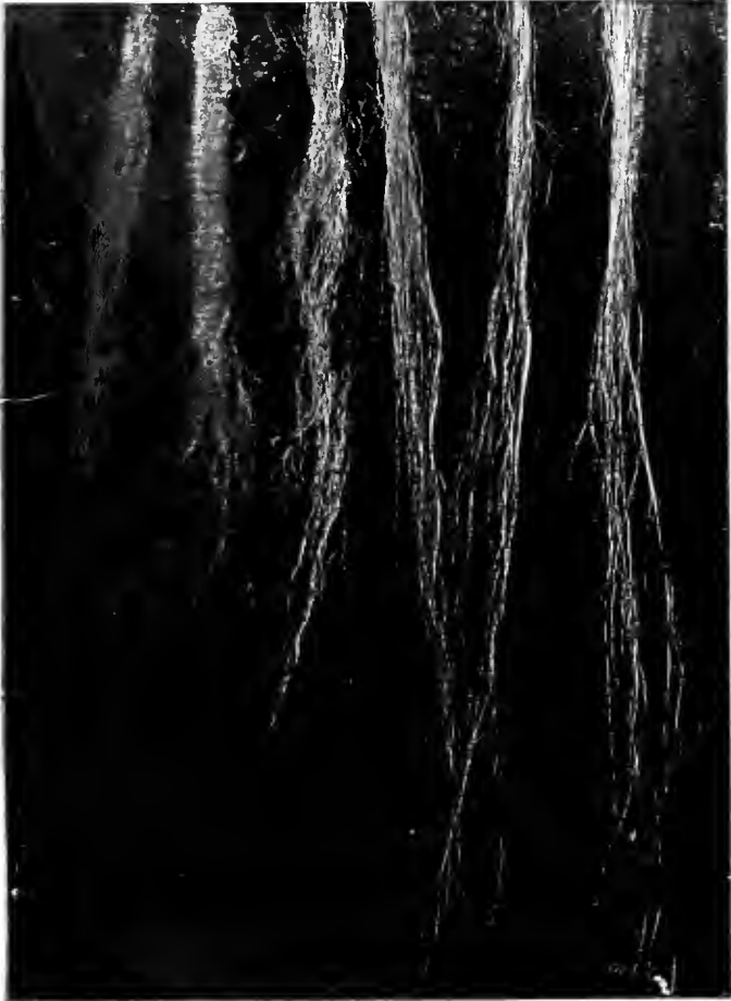
Fig. 3. Untwisted linen yarn—three threads at right; and cotton yarn—three threads at left. Mag. 8x.
